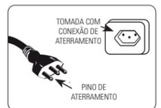
FIGURA 8.1 - CONEXÃO DO PLUGUE A TOMADA (MONOFÁSICO)
